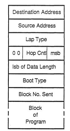
The boot response frame is used by the master station to reply to the slave station with specific boot blocks.
