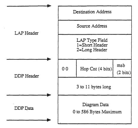
**Receive Buffer Packet Data Structure**
