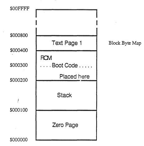
The ROM boot code is placed at \$00200 by the firmware after the user initiates a boot sequence.
