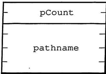
The diagram shows a parameter block structure. It consists of two main sections. The first section starts at offset \$00 and contains a field labeled 'pCount'. The second section starts at offset \$02 and contains a field labeled 'pathname'. The 'No.' column indicates that there is 1 parameter in the second section. The 'Size and type' column describes each field: 'pCount' is a 'Word input value (minimum = 1)' and 'pathname' is a 'Longword input pointer'.
