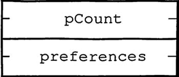
A diagram showing a parameter block structure. It consists of two adjacent words. The first word, starting at offset \$00, is labeled 'pCount'. The second word, starting at offset \$02, is labeled 'preferences'. The number '1' is placed between the two words, indicating the total number of parameters in the block.
