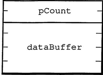
A diagram showing a parameter block structure. It consists of two rows. The first row is labeled 'pCount' and is associated with offset '\$00'. The second row is labeled 'dataBuffer' and is associated with offset '\$02'. To the right of the 'dataBuffer' row, there is a '1' indicating the number of longword pointers.
