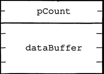
A diagram showing a parameter block structure. It consists of two rectangular boxes stacked vertically. The top box is labeled 'pCount' and is positioned between the offset markers '\$00' and '\$02'. The bottom box is labeled 'dataBuffer' and is positioned below the '\$02' marker. To the right of the 'dataBuffer' box, there is a '1' and the text 'Longword input pointer'. The 'pCount' box is associated with the 'Word input value (minimum = 1)' description.
