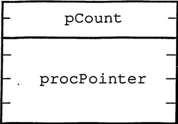
A diagram showing a parameter block structure. It consists of a vertical rectangle divided into two sections. The top section is labeled 'pCount' and is bounded by horizontal lines at offsets \$00 and \$02. The bottom section is labeled 'procPointer' and is bounded by horizontal lines at offsets \$02 and \$06. To the right of the 'procPointer' section, the number '1' is written, indicating the number of longword pointers in that section.
